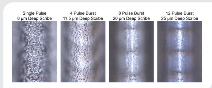
Figure 3. The excellent machined surface quality that can be achieved with picosecond UV laser processing is seen in these images. The advantage of higher pulse count bursts is plainly evident here.
