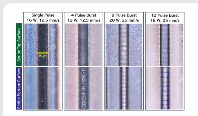
Figure 2. Microscope images showing tops and floors of 25 µm deep grooves. These show a steady improvement in scribe quality as the number of pulses in the burst increases.
