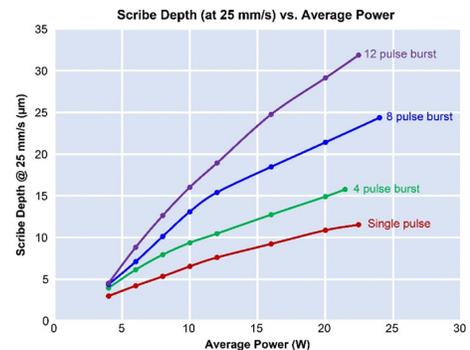
Figure 1. Scribe depth at 25 mm/s net speed as a function of power for single pulses and various burst configurations (4-12 burst sub-pulses). Clearly pulse bursts improve ablation rates.
